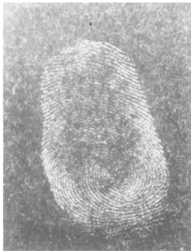
FIG. 1—Greasy fingerprint fluorescence under UV light after simple spray treatment (photographed with Kodacolor film, ISO 100, exposure time 3 s at f-stop 22).
